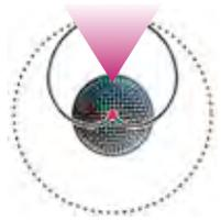
A third effect, known as the "proximity effect" is that the microphone will emphasize the low frequency components of any source that is very close to the diaphragm. Many cardioid microphones have a built in filter switch to compensate for proximity. Bidirectional mics also exhibit this phenomenon.
